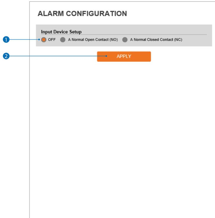
1 **Input device setup** - Select input device type from OFF / N.O. / N.C.
